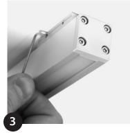
Secure slider to plate with hex key.
